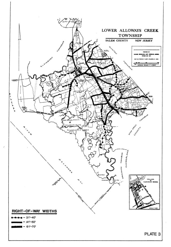
In most cases, no roadway should have a right-of-way width less than fifty (50) feet. These roads should perform only the basic local traffic function of providing access to abutting properties; no through traffic should be part of the traffic flow. When a roadway is called upon to handle through-traffic volumes, such as a connector road between major highways or residential concentrations, the required right-of-way should be at least sixty (60) feet and sometimes more.
